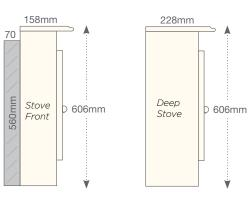
The FocusFlame Stove Front can be supplied to fit into a 3" rebate or as a free standing Deep Stove version where hearth space allows.
