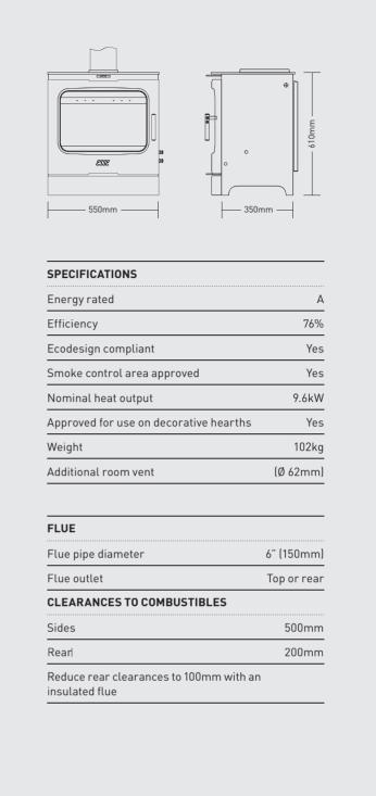
Designed for larger spaces, the ESSE 775 creates an impression as well as a powerful heat source. The generous, deep fire bed adds visual drama, while our efficient stove convection system keeps temperatures toasty.
