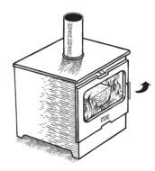
5. After 15 minutes the heat will be sufficient to create a draught through the flue. Position controls to the desired burn rate.
