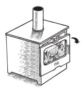
**4.** As the fire starts fully open all airway and filter controls.
