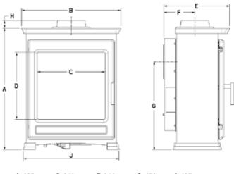
A 625mm C 349mm E 340mm G 452mm J 495mm B 511mm D 344mm F 161mm H39
