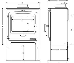
A 588mm C 260mm E 352mm G 111mm 1 500mm K 250mm B 528mm D 249mm F 310mm H 478mm J 330mm
