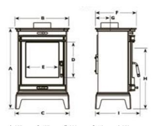
A 637mm C 427mm E 260mm G 113mm I 353mm B 430mm D 275mm F 326mm H 507mm
