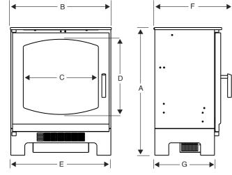
A 595mm C 352mm E 466mm G 307mm B 471mm D 350mm F 359mm WARNING BFM Europe Limited is a Gas Safe Registered company. We recommend all our gas stoves are installed by a Gas Safe Registered engineer, and all Multifuel or Wood burning stoves are fitted by a HETAS registered engineer, in accordance with our installation and user manuals.
