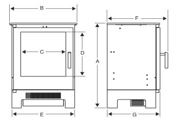
A 582mm C 288mm E 400mm G 337mm B 430mm D 304mm F 389mm
