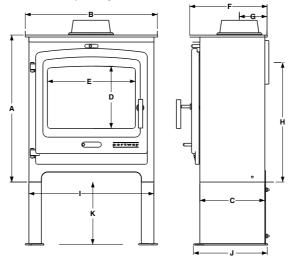
A 588mm C 260mm E 352mm G 111mm I 500mm B 528mm D 249mm F 310mm H 478mm J 310mm K 150/300mm High/Low Legs
