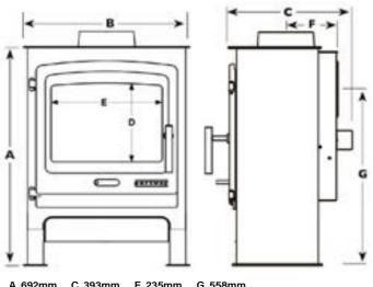
A 692mm C 393mm E 235mm G 558mm B 523mm D 357mm F 160mm
