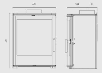
Clearance to combustibles to the top is 400mm and 300mm to the sides, clearance to non-combustibles is 50mm. Please refer to the installation instructions for more info.
