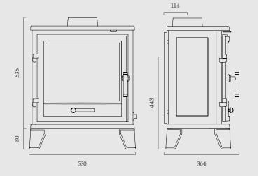
$\label{lem:clearance} Clearance\ to\ combustibles\ is\ 600mm,\ clearance\ to\ non-combustibles\ is\ 50mm.$   $Please\ refer\ to\ the\ installation\ instructions\ for\ more\ info.$
