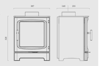
Clearance to combustibles is 600mm, clearance to non-combustibles is 50mm.
