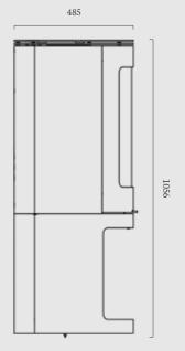
Clearance to combustibles is 50mm to rear and 250mm to sides, clearance to noncombustibles is 50mm. Please refer to the installation instructions for more info.
