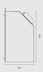
Minimum clearance to combustibles: Rear - back of chamber must be non-combustible. Sides - 600mm. Please refer to the installation instructions for more info.
