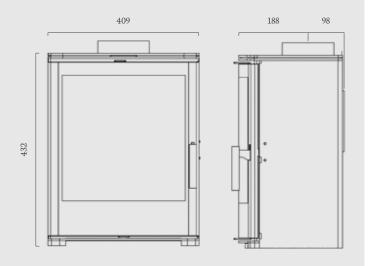
See page 43 for Prime and Supreme Leg dimensions. Clearance to combustibles to the top is 400mm and 300mm to the sides, clearance to non-combustibles is 50mm. Please refer to the installation instructions for more info.
